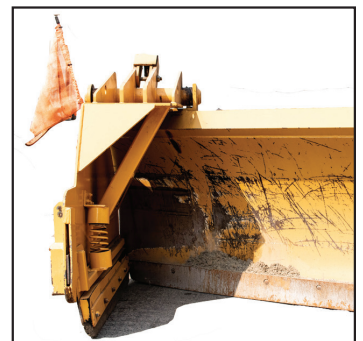
Close-up of a snow gate
